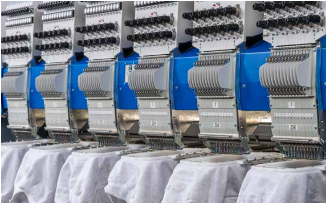
ZSK Racer 6 Head in Tubular Mode Embroidering on Sweatshirts
