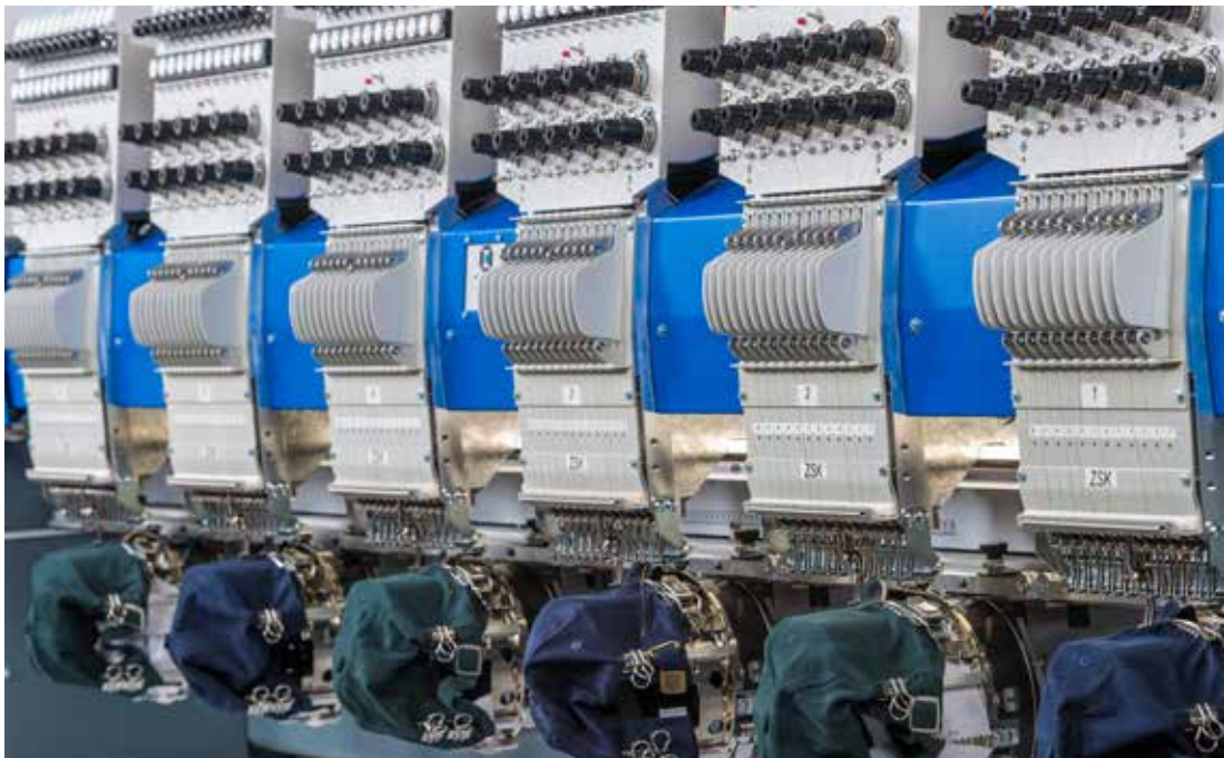
ZSK Racer 6 Head in Cap Mode Embroidering on Hats
