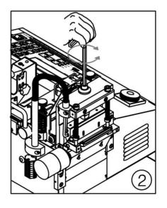
③ Take off the heater after unscrewing the fixing bolt by 4~5mm-wrench. (Install new upper knife and assemble it again vice versa.)
