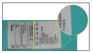
Sometimes you can see a label, one side is sealed well, but the other side is not sealed well.
