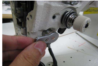
5: Loose screw of Hand switch
