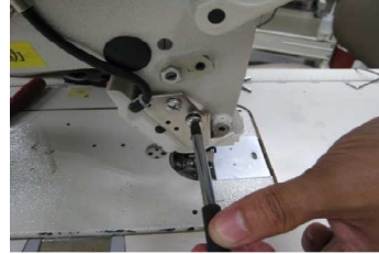
5: Loose screw of Hand switch
