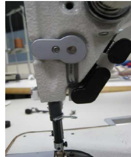
6: Cable must follow arm channel
