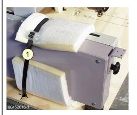
• Remove the lashing straps (1) that secure the control cabinet and machine to **the pallet**.
