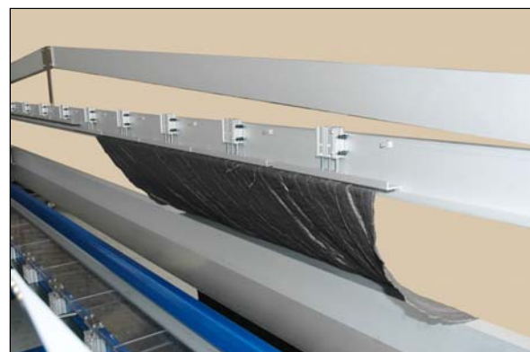
Figure 37 Putting curtains with finished pocket aside
