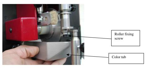
Replace the roller and repeat the above operation, making sure that the knobs have been securely fastened.
