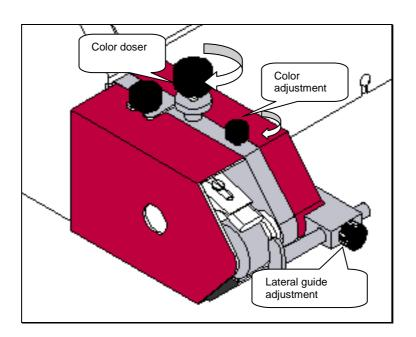
To adjust the position and pressure of the dye applicator brush, loosen the corresponding knob, manually adjust the position of the brush and tighten the knob once more.
