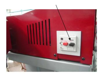
The green warning LED "TENSION" (Voltage) lights up on the control panel to show that the machine is powered. (see below picture)
