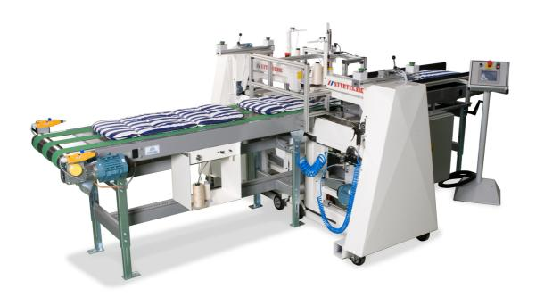
Working procedure: The cushions are placed on a conveyor between two HECTOR standard machines, placed opposite each other. Via a photocell the cushions are fed into position and the tufting takes place automatically.
