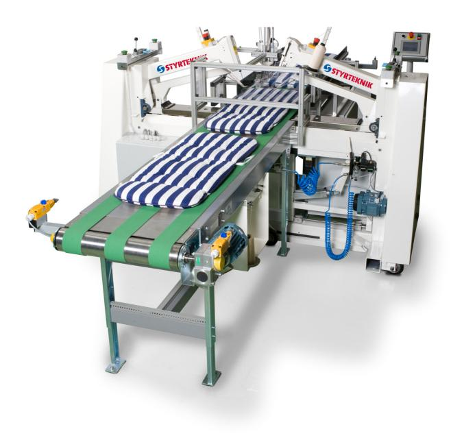
Working procedure: The cushions are placed on a conveyor between two HECTOR standard machines, placed opposite each other. Via a photocell the cushions are fed into position and the tufting takes place automatically.
