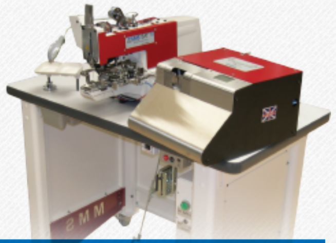
MK 11 mounted to work in tandem with an MMS BAT 16
