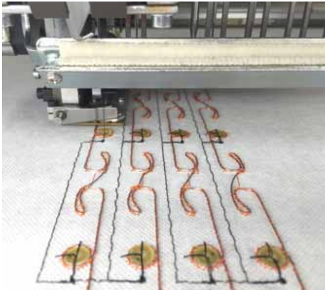
RFID antennas placed and fixed by embroidery.
