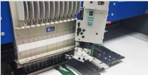
Fig.: Cording Device EP 1.2 at ZSK F-Head
