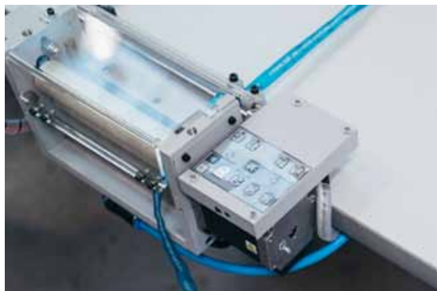
Fig.: Automatic Pull Through Device of ROLL2BASKET
