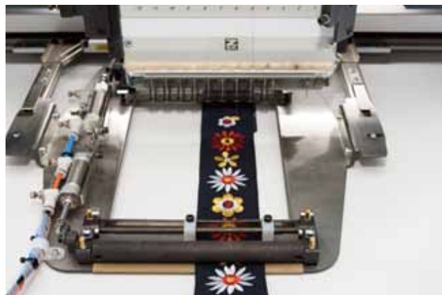
Fig.: Automatic Clamping Frame of ROLL2BASKET
