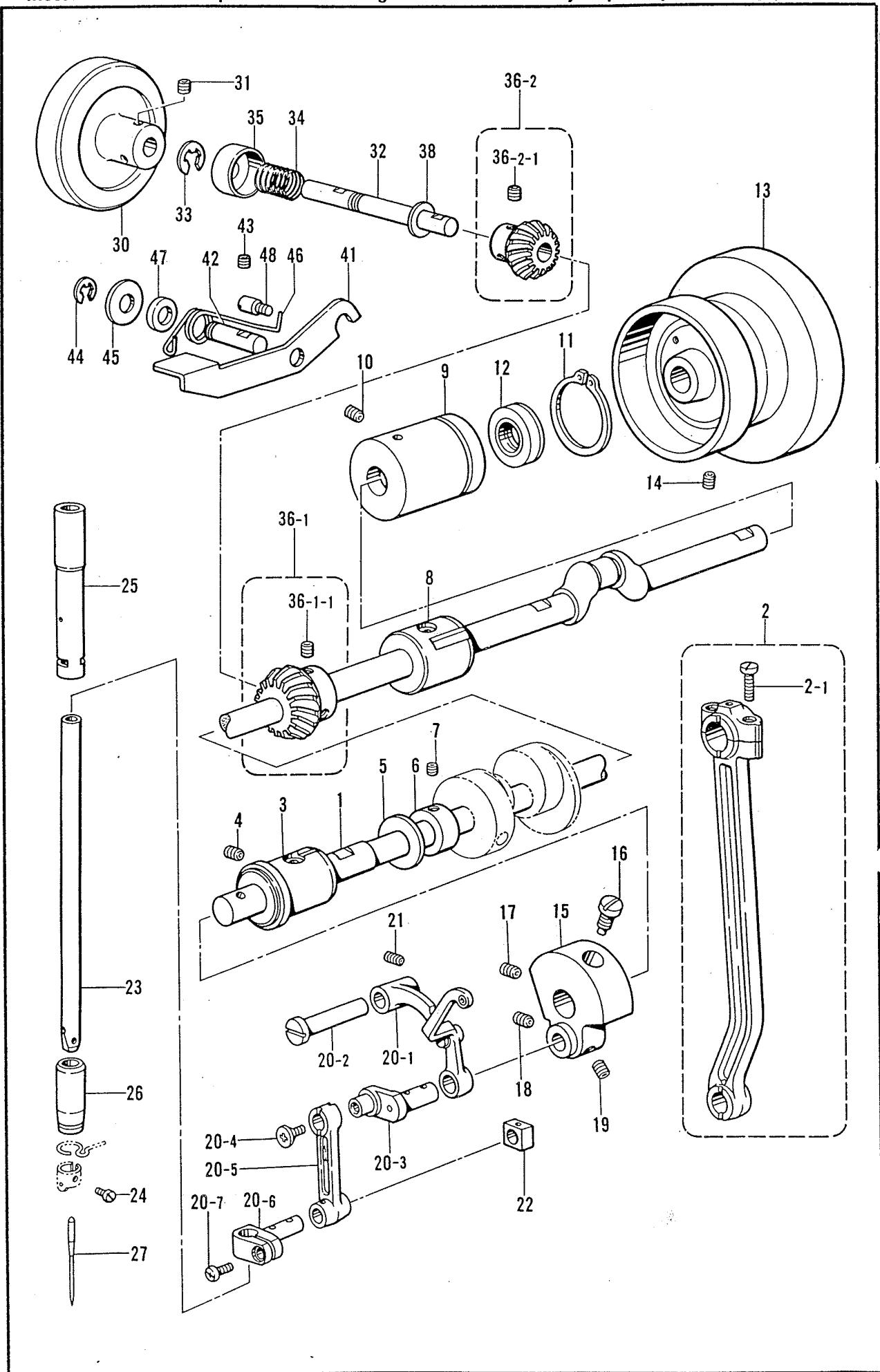
UPPER SHAFT AND NEEDLE BAR MECHANISM / OBERE WENGE UND NÄDELSTABMECHANIK /
