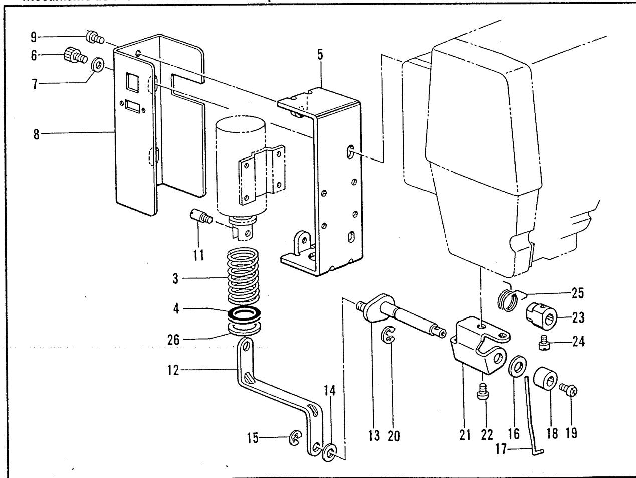
M. 糸切れ感知関係 / Thread breakage detector mechanism / Fadenbruchfühler /
