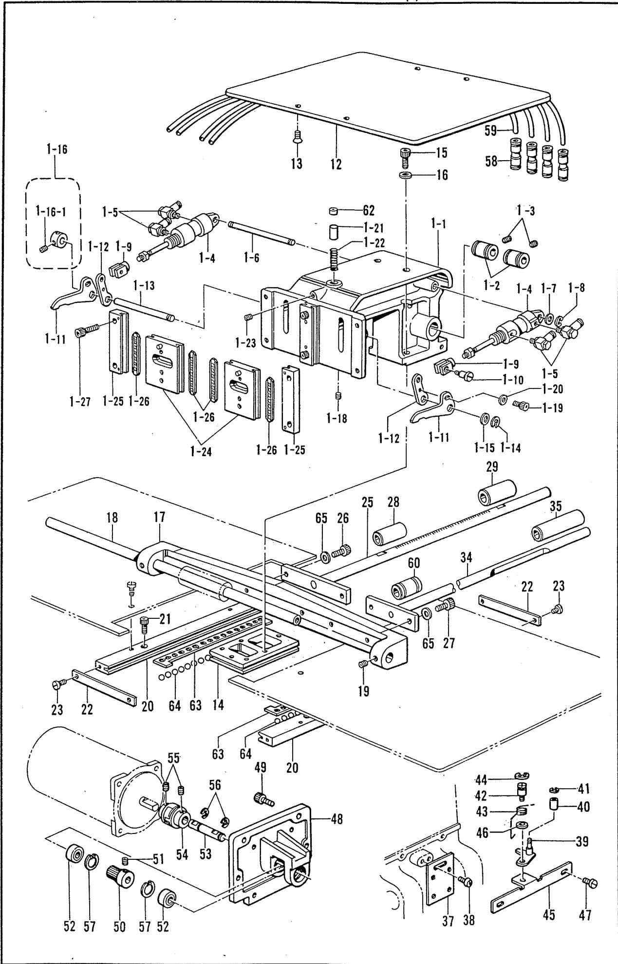
D1. 送り関係 / Feed mechanism (1) / Transportvorrichtung (1) /
