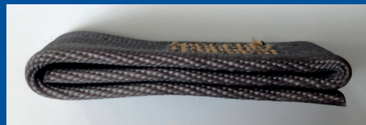
six-ply sewing for seatbelt
