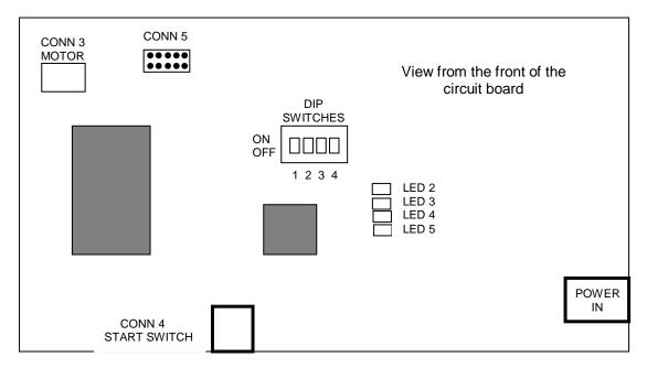
The DIP switches are located in the centre of the circuit board. These can be switched to achieve different operating modes as follows : (note – disconnect the power to the machine before opening the cover to make the adjustments).
