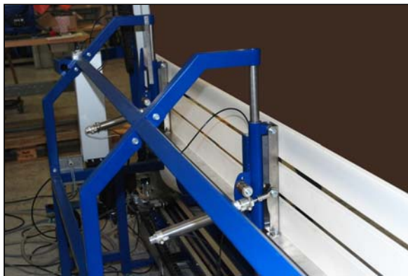
Figure 13 Cylinders for folding the work table
