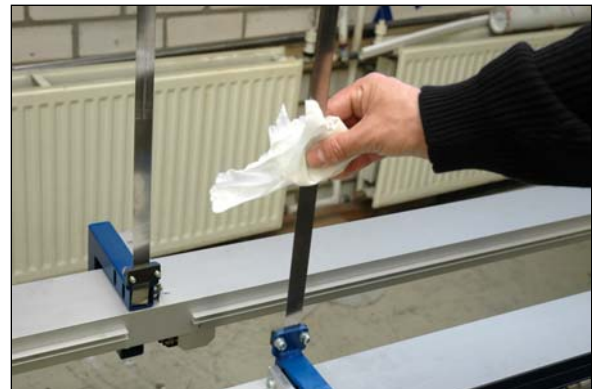
Figure 27 Cleaning the lifting straps
