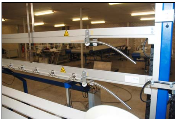
Figure 4 Spring-loaded fabric clamps
