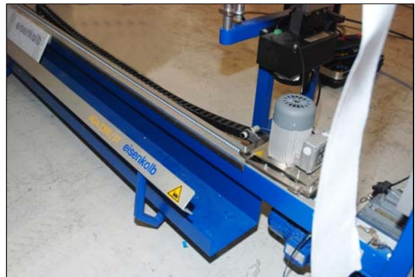
Figure 5 Fabric clamp, fabric catcher and cutter carriage
